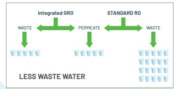
PENTAIR GRO-75EN HIGH EFFICIENCY integrated GRO MEMBRANE : 50% recovery 100L Osmosis water = 200 litre effectively used
