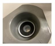
Ensure the internal seal and external seals are in position.
